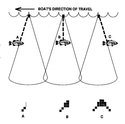
Very small fish probably will not arch at all. Medium sized fish will show a partial arch, or a shape similar to an arch if they're in deep water. Large fish will arch, but turn the sensitivity up in deeper water to see the arch. Because of water conditions, such as heavy surface clutter, thermoclines, etc., the sensitivity sometimes cannot be increased enough to get fish arches.
